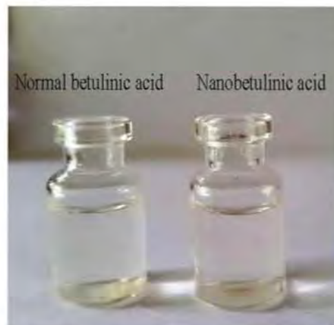
Figure 8. The solubility test of normal betulinic acid and nanobetulinic acid in ethanol solvent.
